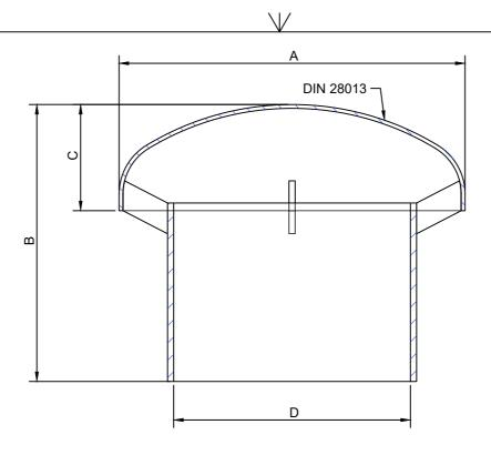
Standard type: Material: Galvanised steel body
